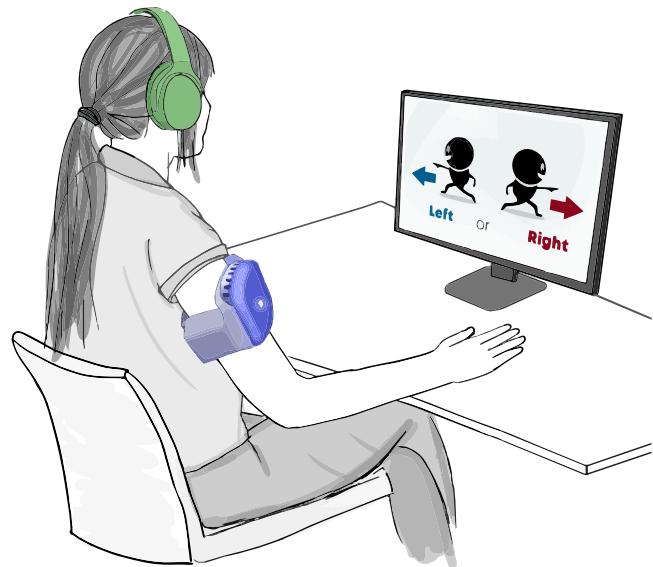
Fig. 4. Setup for the ST. The MiSMT device is worn on the upper arm of the non-dominant side, and the participant wears noise-cancelling headphones.
